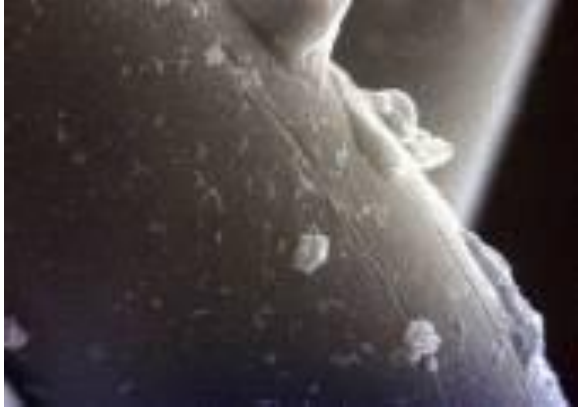
Figure 2. Catcher-mesh with single discrete particles SEM x1000
