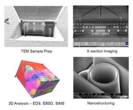
**Figure 2.** Applications such as (a) TEM sample preparation (b) preparation of cross-sections and (c) 3D analysis will greatly benefit from the increased current that is maximally available. At the same time no precision is lost and even delicate nanopatterning tasks may be performed (d).
