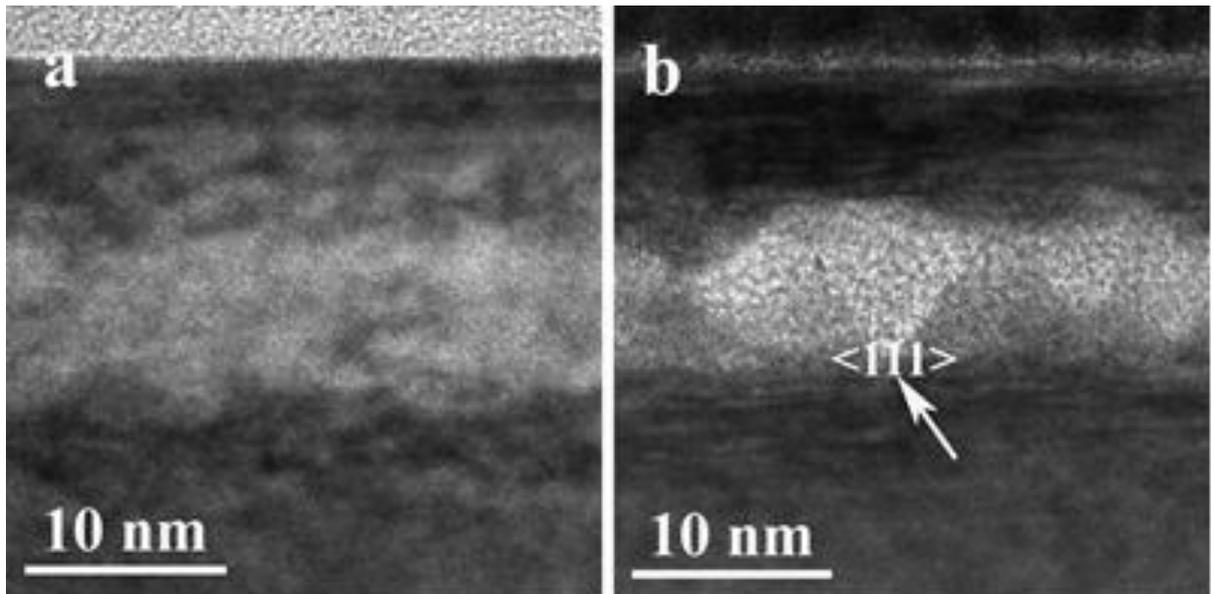
**Figure 1.** HREM images of (001) diamond (a) after implantation with fluence  $3 \times 10^{14}$  ions/cm<sup>2</sup> and (b) after HPHT annealing.
