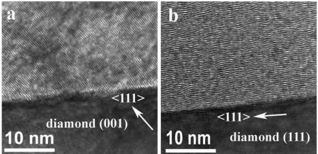
**Figure 2.** HREM images of the (a) (001) and (b) (111) diamond samples implanted with fluence  $10^{15}$  ions/cm<sup>2</sup> and HPHT annealed at 1200 °C and 4 GPa.
