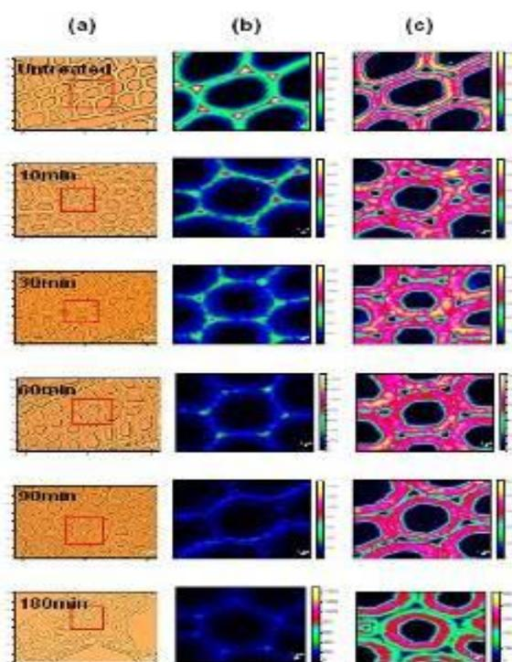
**Figure 2.** Bright field images of poplar cross-sections showing selected area (*red rectangle*) for Raman imaging (a); Raman images showing the distribution of main components within cell walls at various pretreatment time by integrating from 1570 to 1680  $\text{cm}^{-1}$  (b, lignin) and 2850-2920  $\text{cm}^{-1}$  (c, carbohydrate).
