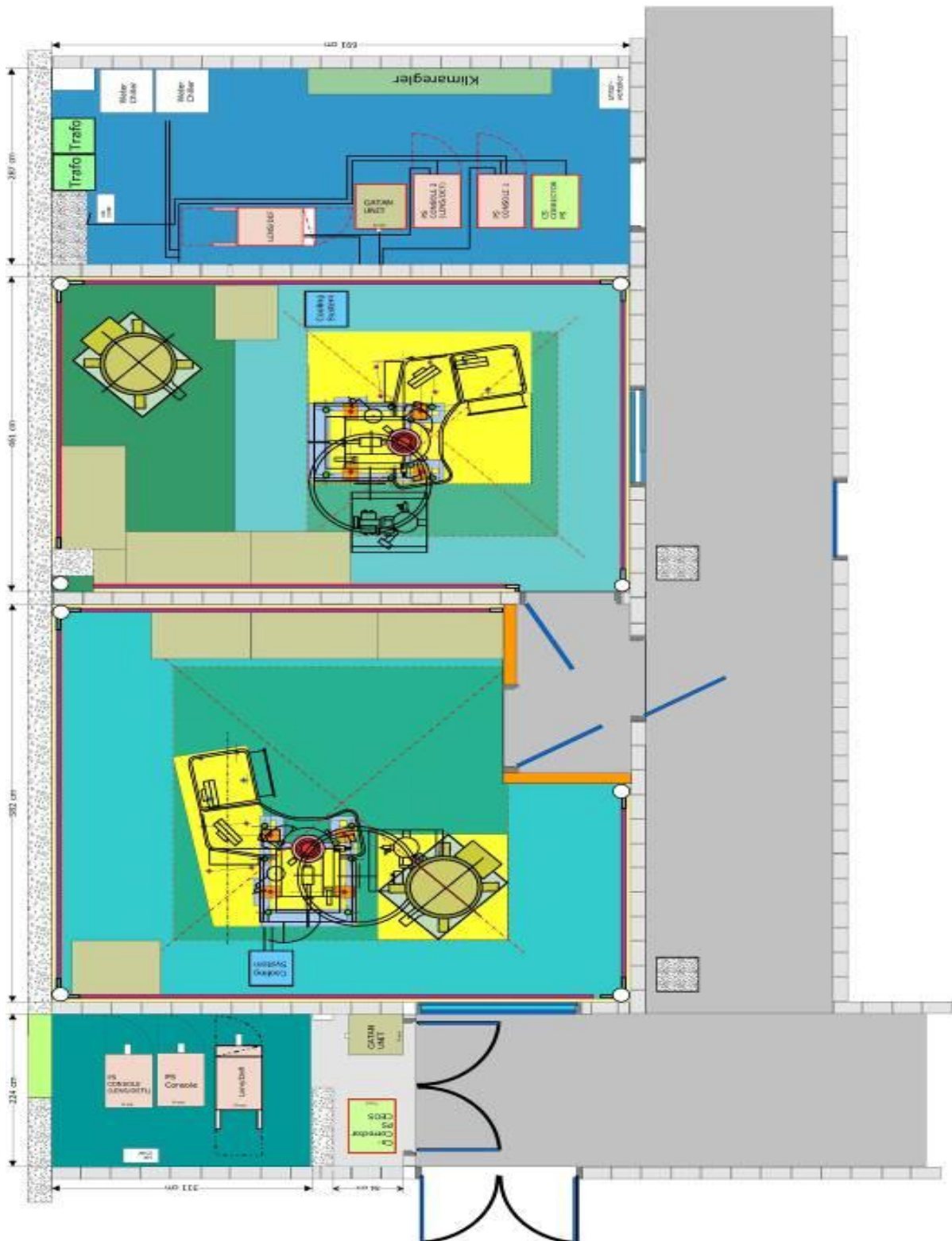
Figure 1. Room design for the new JEOL JEM-ARM 200F microscopes at the Stuttgart Center for Electron Microscopy
