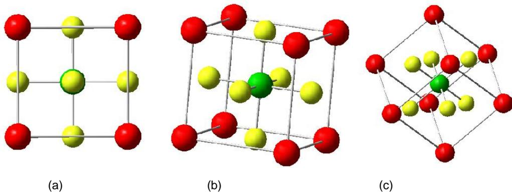
**Figure 1.** Structure of strontium titanate (red: strontium, green: titanium, yellow: oxygen); Simulations in the following figures conducted with a strontium titanate specimen in [001]-orientation (a).
