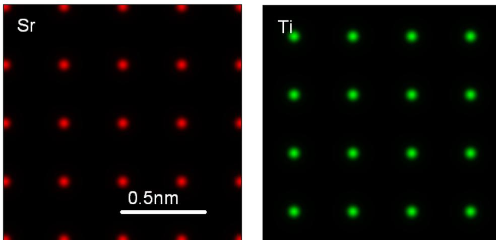
**Figure 2.** Simulation of Sr-L and Ti-K signals in elemental maps of SrTiO<sub>3</sub> assuming an aberration corrected STEM. The size of the simulated image is 128x128 pixels [3].
