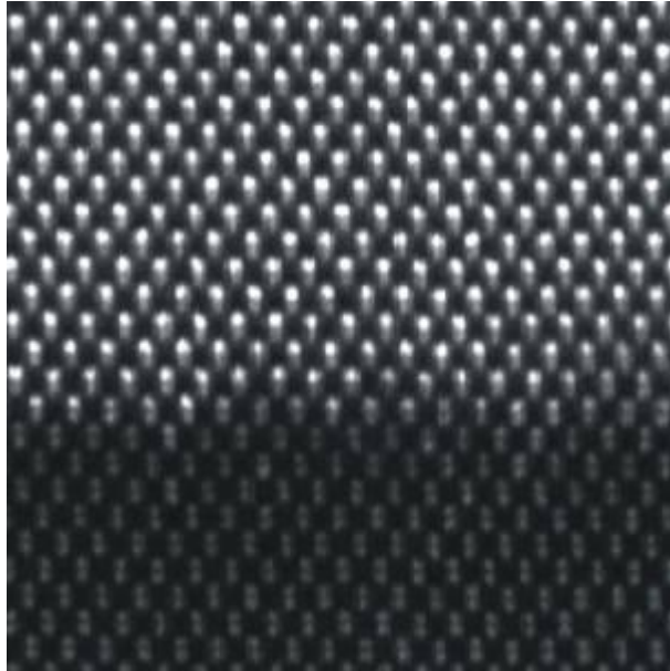
Figure 1. Representative HAADF-image of the GaP/Si-interface (The width of the scalebar is 1 nm).
