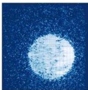
Figure 3. Single frame with 1 ms exposure time at a primary electron energy of 300 keV showing a Bragg disc of a diffraction pattern. The signal outside the disc is not noise but originates from primary electrons which are scattered at the sample, while the structure inside the disc is due to dynamical scattering.
