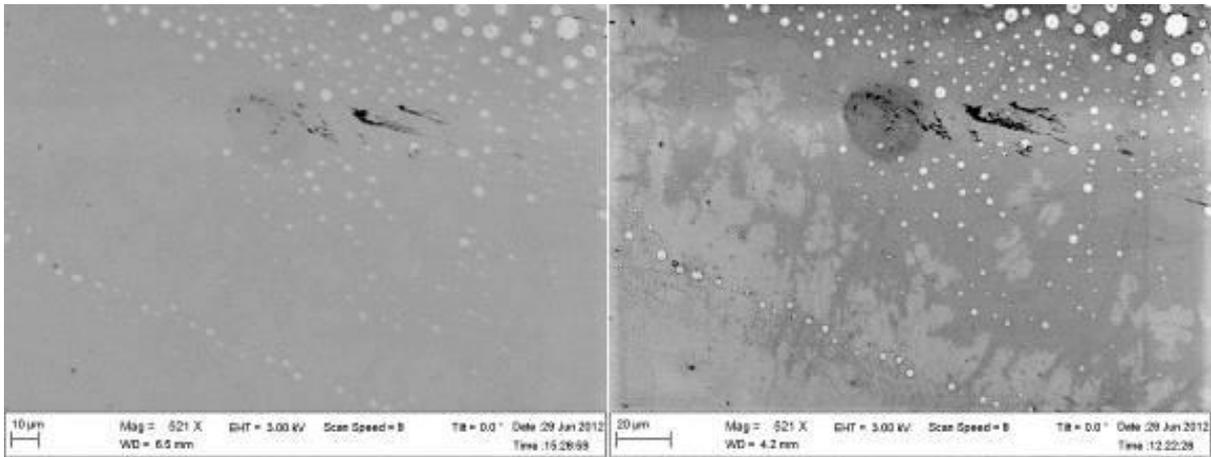
**Figure 2.** Two BSE images taken at 3 keV primary beam energy and identical microscope and readout conditions. The left image was taken with a standard geometry detector while the right image is from a detector with optimized entrance window and geometry and shows a highly improved contrast.
