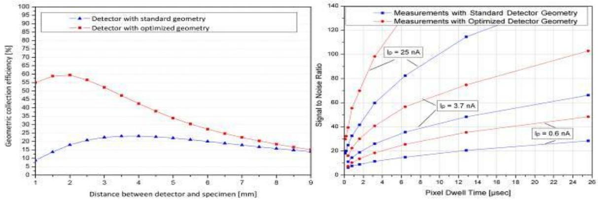
**Figure 1.** a) Calculated geometric collection efficiency for different detector geometries. 100 % correspond to a solid angle of  $2\pi$ . b) Measured Signal to noise ratio as a function of pixel dwell time for three different primary beam currents. The new detector with optimized geometry shows a large increase of the SNR.
