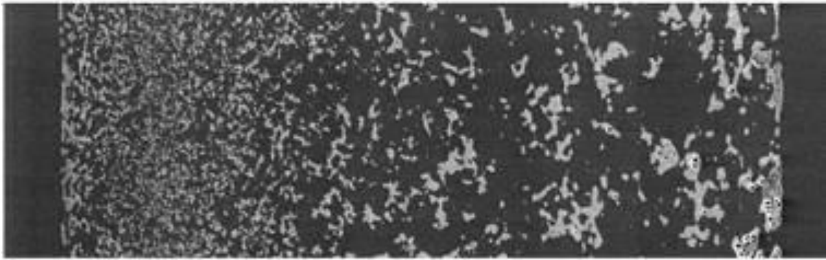
Figure 1. Cross-section of the membrane DuraPES ® 600 (image width: 174 μm).
