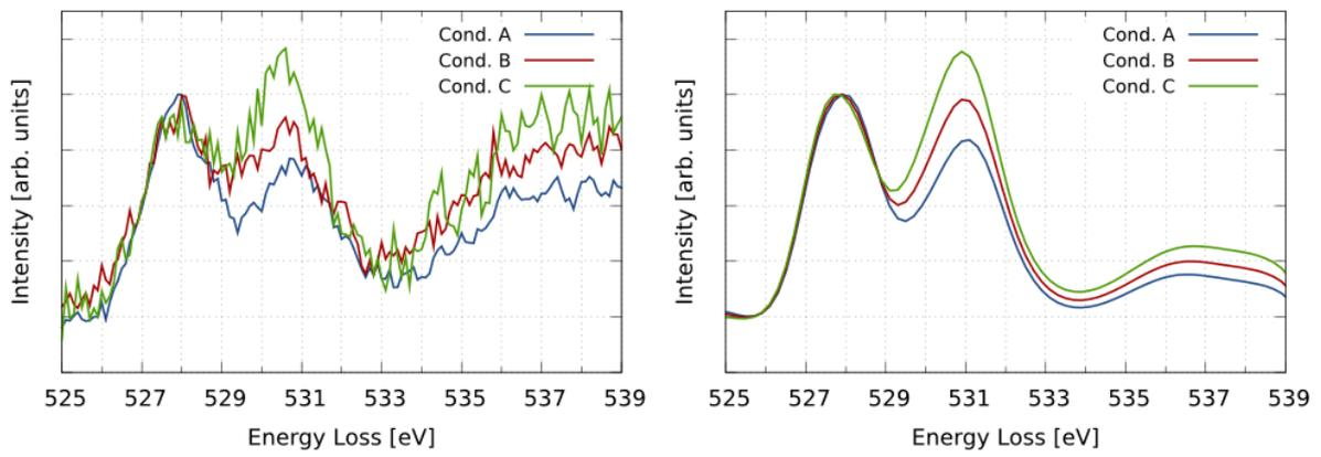
**Figure 2.** Left: acquired O K-edge ELNES under three different channelling conditions. Right: corresponding calculated spectra. All spectra were normalised to the first peak to facilitate comparison.
