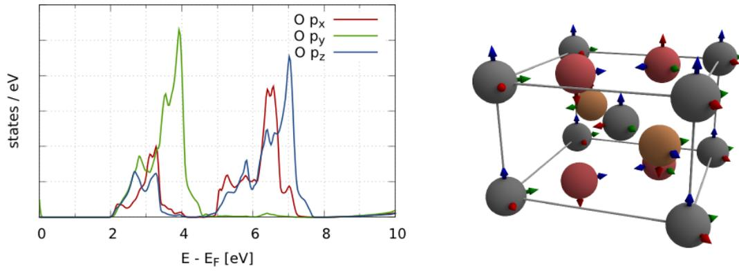
**Figure 1.** Left: calculated partial DOS of p-character for oxygen. Right: unit cell of rutile (grey: titanium, red/brown: oxygen). The arrows show the directions of the corresponding  $p_x$ -,  $p_y$ - and  $p_z$ -orbitals.
