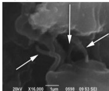
**Figure 4.** SEM image of the fracture surface after tensile testing of PEX nanocomposite containing 3% MWCNTs.
