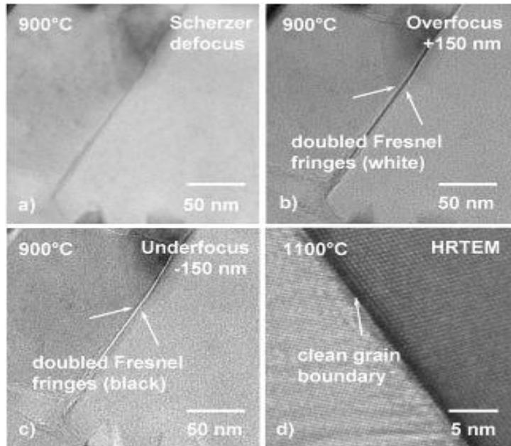
**Figure 1.** Defocus series of a spinel-spinel grain boundary. The material was sintered at 900°C [a,b,c] and 1100°C [d]. The double fringes occurring at 900°C indicate a twice changing mean inner potential which was interpreted as a wetting of the grain boundary. At higher temperatures no wetting was observed.
