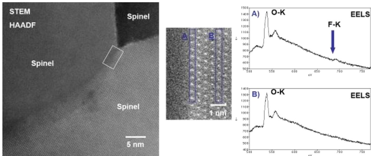
**Figure 2.** HR-STEM image of a spinel-spinel grain boundary. When applying the defocus technique double Fresnel fringes occurred but even in highest magnification no wetting could be shown. Instead, by using STEM EELS techniques, an incorporation of fluorine in the first two atomic layers was observed at a sintering temperature of 900°C.
