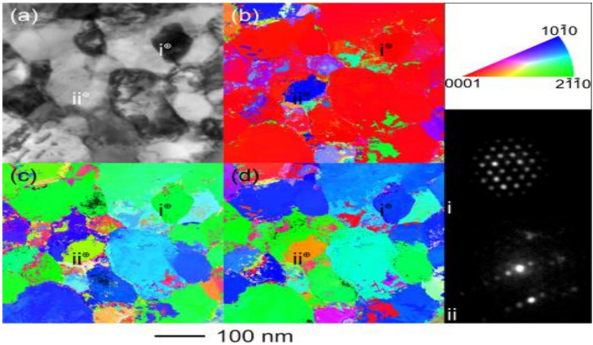
**Figure 1.** Automated crystal orientation mapping of AlN along the basal view. (a) Virtual bright field image. Orientation map along the out-of-plane z-direction (b), and two in-plane directions (c) x-direction, (d) y-direction. (Right) Color code of the stereographic triangle (hexagonal point group:  $6mm$ ) for all three maps. Diffraction patterns of area i) and ii).
