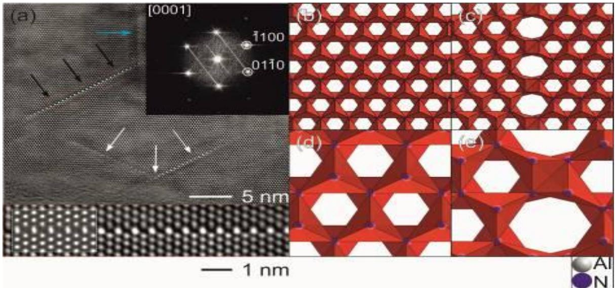
**Figure 2.** (a) HRTEM micrograph along the  $[0\ 0\ 0\ 1]$  zone axis with inserted FFT. Arrows mark the stacking mismatch boundaries. The enlarged panel at the bottom shows a stacking mismatch boundary with a simulation as inset (objective lens defocus | specimen thickness) of  $(-45\ \text{nm} \mid \sim 5.5\ \text{nm})$ . Schematic for the defect-free bulk structure (b) and the structure at the SMB (c) along the  $[0\ 0\ 0\ 1]$  zone axis. (d) and (e) corresponding enlarged views.
