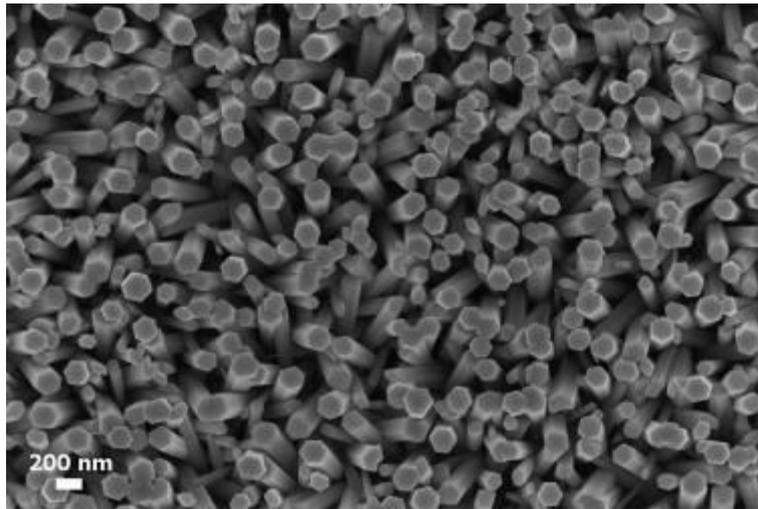
**Figure 1.** FESEM image of Cr-doped ZnO nanowires (top view)
