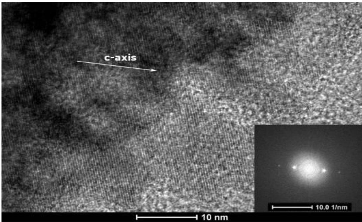
**Figure 2.** Bright field TEM image of a single Cr-doped nanowire. Inset: FFT of the image showing that the nanowire grows along the (002) direction.
