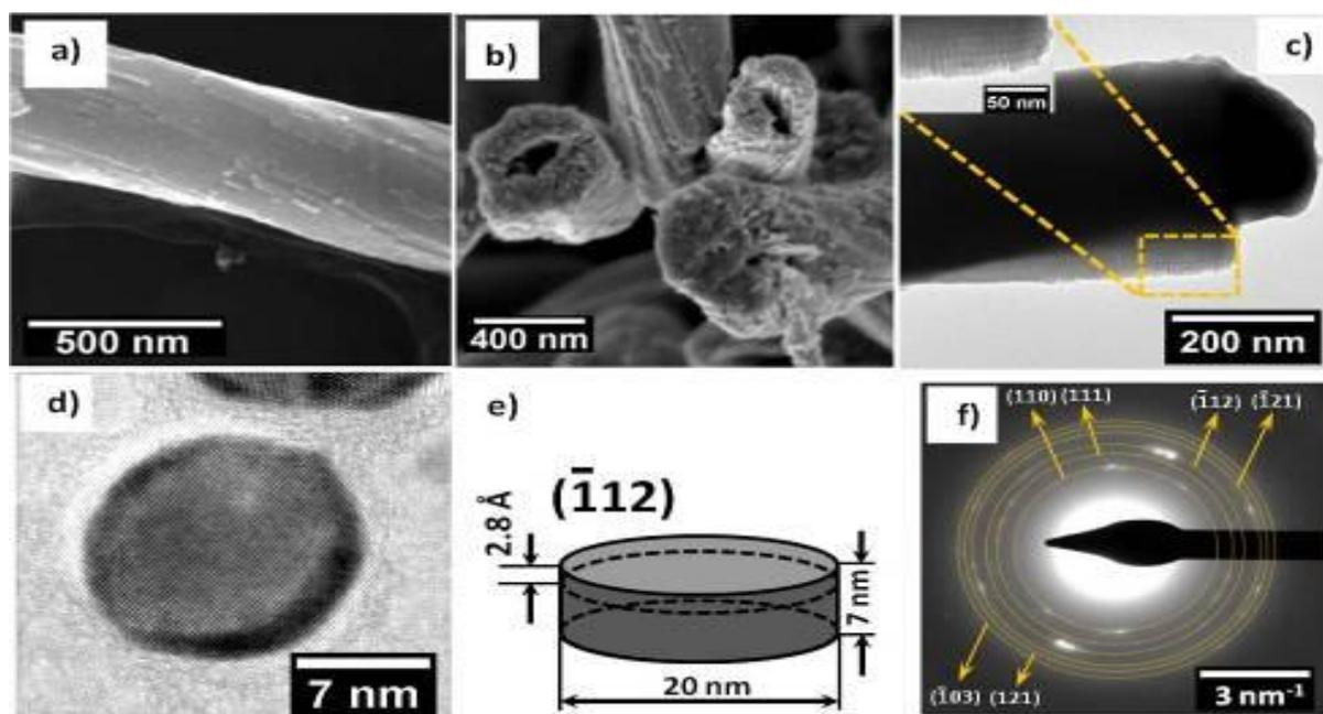
**Figure 2.** (a) Side-view and (b) top-view SEM images of  $\text{Ag}_2\text{S}$  nanodisk supercrystals; (c) TEM image showing stacked nanodisks; (d) HRTEM and (e) schematic representation of a single  $\text{Ag}_2\text{S}$  ND; (f) indexed SAED pattern of  $\text{Ag}_2\text{S}$  ND supercrystals, which shows a strong  $(\bar{1}12)$  texture (Miller indices correspond to bulk monoclinic  $\alpha$ - $\text{Ag}_2\text{S}$ /acanhite).
