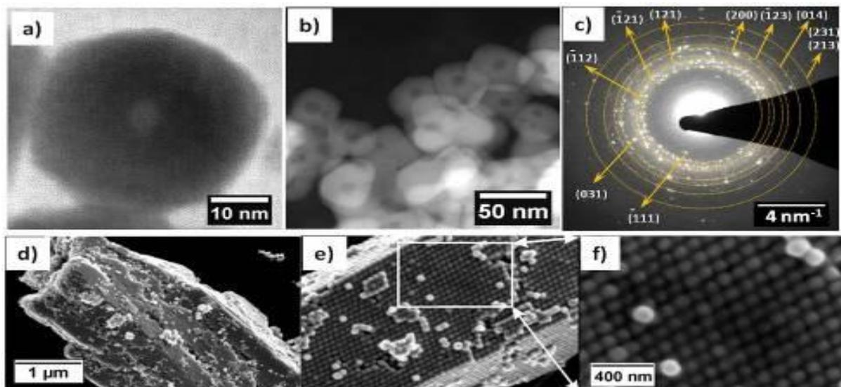
**Figure 1.** (a) HRTEM and (b) HAADF-STEM images of single  $\text{Ag}_2\text{S}$  HSs; (c) indexed SAED pattern of  $\text{Ag}_2\text{S}$  supercrystals (Miller indices correspond to bulk monoclinic  $\alpha$ - $\text{Ag}_2\text{S}$ /acanhite); (d) overview SEM image and (e,f) detail SEM images of  $\text{Ag}_2\text{S}$  hollow sphere supercrystals showing the dense packing of hollow spheres.
