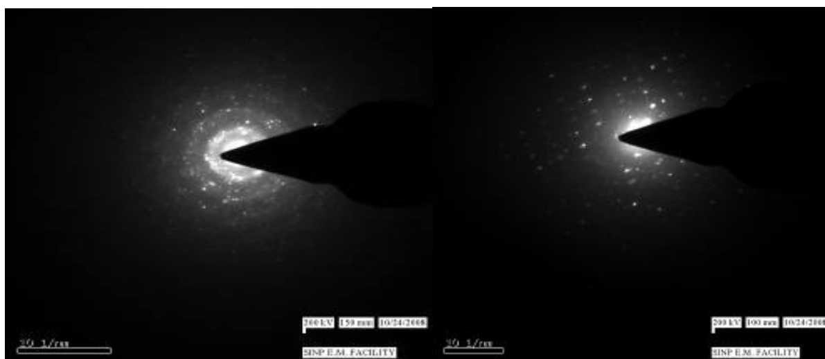
Figure 1. Diffraction rings seen by 200 kV Transmission Electron Microscopy of orthorhombic PNO (left figure) and of rhombohedral PNO (right figure).
