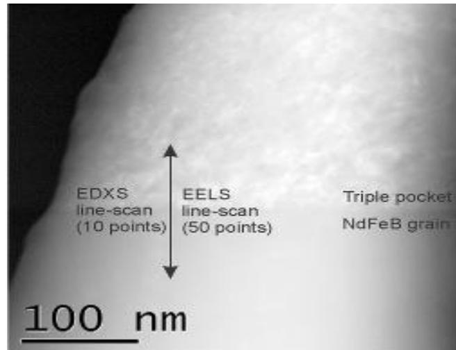
**Figure 1.** HAADF-STEM image of a Nd–Fe–B grain adjacent to a triple pocket. The EDXS and EELS line-scans are marked on the image.
