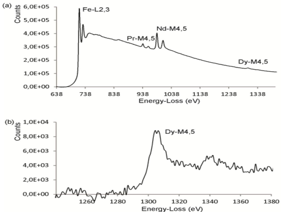
**Figure 2.** Background-subtracted (a) averaged EELS spectrum acquired from the Nd–Fe–B grain adjacent to the TP and (b) enlarged Dy-M<sub>4,5</sub> energy-loss region.
