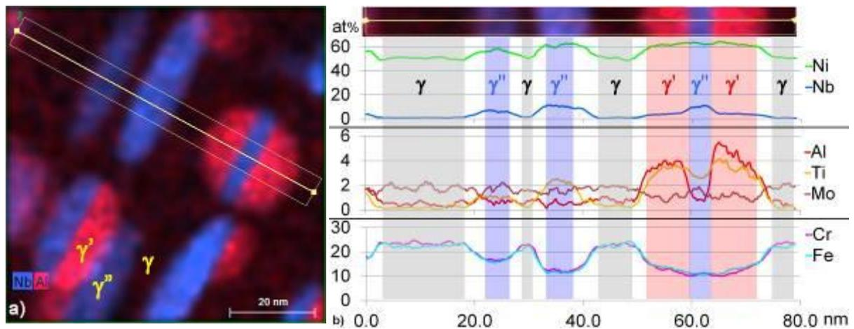
**Figure 2.** a) EDX ChemiSTEM map of Al (red) and Nb (blue) that distinguishes the  $\gamma'$  and  $\gamma''$  precipitates; b) Composition changes along a line scan across the three phases. Notice the unexpected presence of Nb in the  $\gamma'$  phase.
