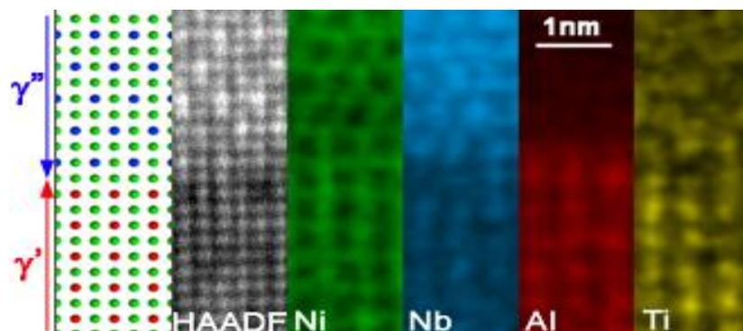
**Figure 3.** EDX ChemiSTEM maps of a  $\gamma'/\gamma''$  interface. The Nb substitute to Al in the  $\gamma'$  phase
