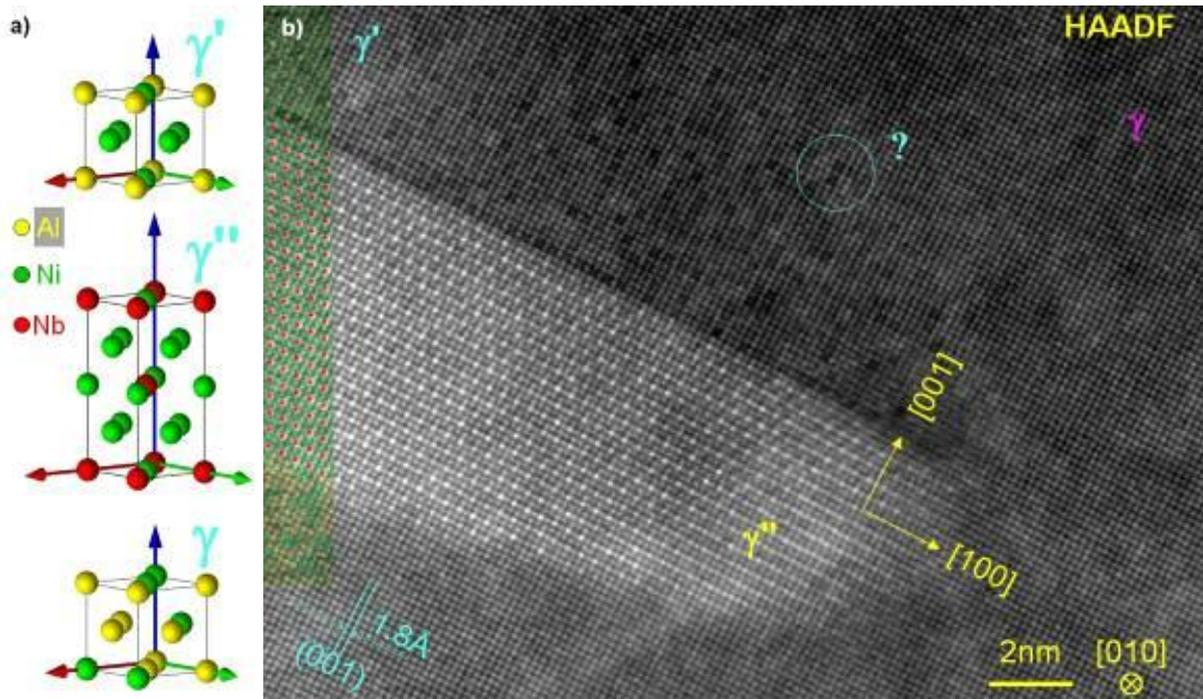
**Figure 1.** a) ball model of the  $\gamma$  matrix and the  $\gamma'$  and  $\gamma''$  phases; b) HAADF high-resolution STEM image of  $\gamma'$  and  $\gamma''$  precipitates in the  $\gamma$  matrix. All interfaces are coherent, but the  $\gamma'/\gamma''$  one as well as the  $\gamma'$  precipitate contain defects at the atom column scale.
