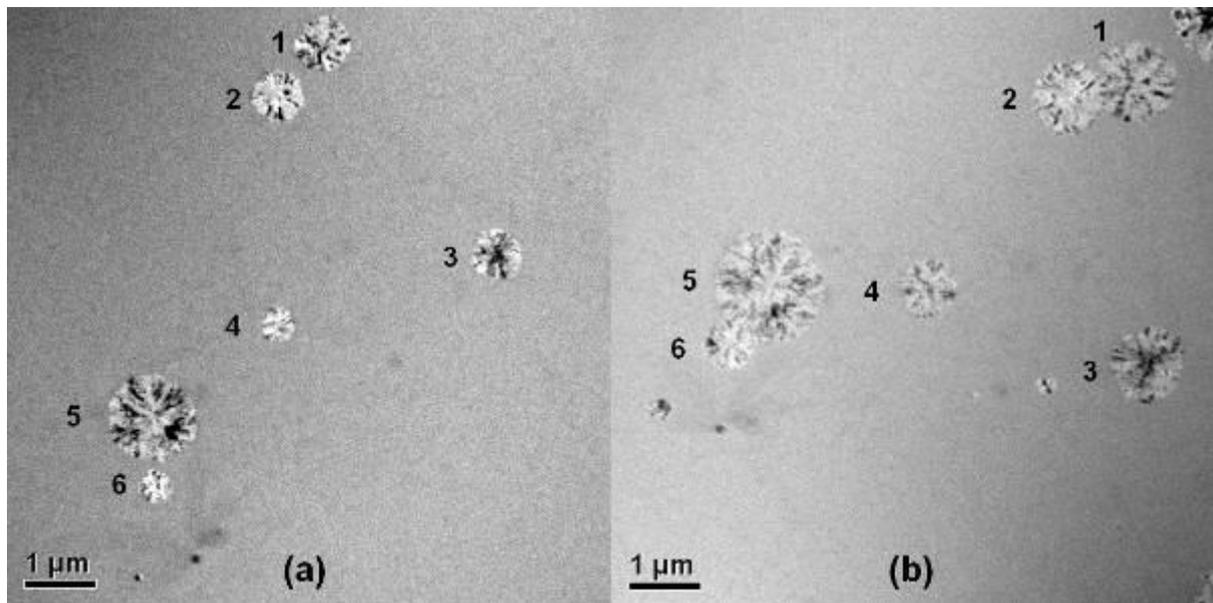
**Figure 2.** (a). Transmission electron microscope brightfield image of crystalline grains in an amorphous Ag<sub>4</sub>In<sub>3</sub>Sb<sub>67</sub>Te<sub>26</sub> layer after 90 min *ex situ* heating in a furnace at 418.15 K. (b). The grains from image (a) after 10 min additional heating (100 min in total) at 418.15 K.
