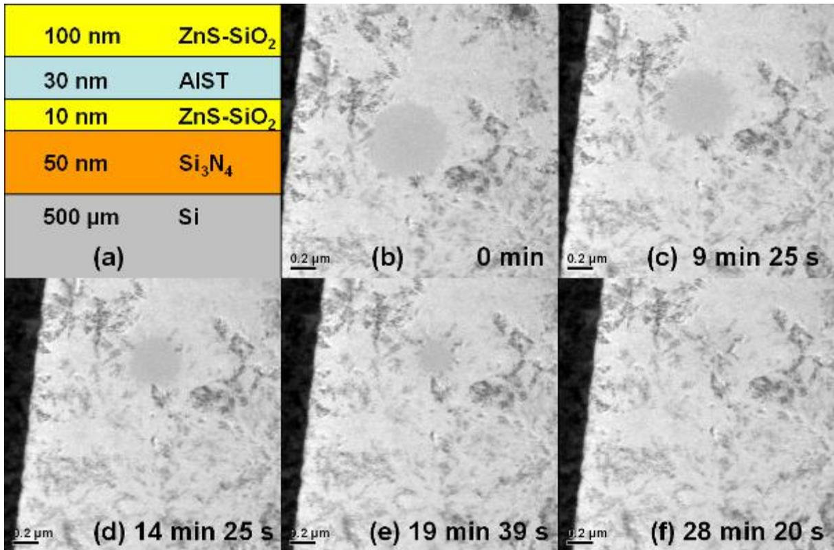
**Figure 1.** (a). Schematic drawing of the multilayer stack on silicon substrate before etching. (b)-(f). Transmission electron microscope brightfield images of an amorphous melt quenched region within a crystalline Ag<sub>4</sub>In<sub>3</sub>Sb<sub>67</sub>Te<sub>26</sub> layer heated *in situ* at 383 K. The displayed time is related to the start of heating [3].
