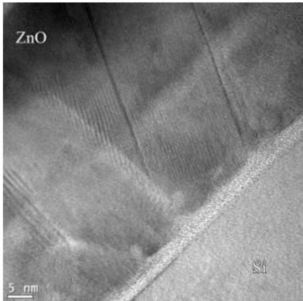
**Figure 1.** BF TEM image of ZnO deposited on (111) Si.
