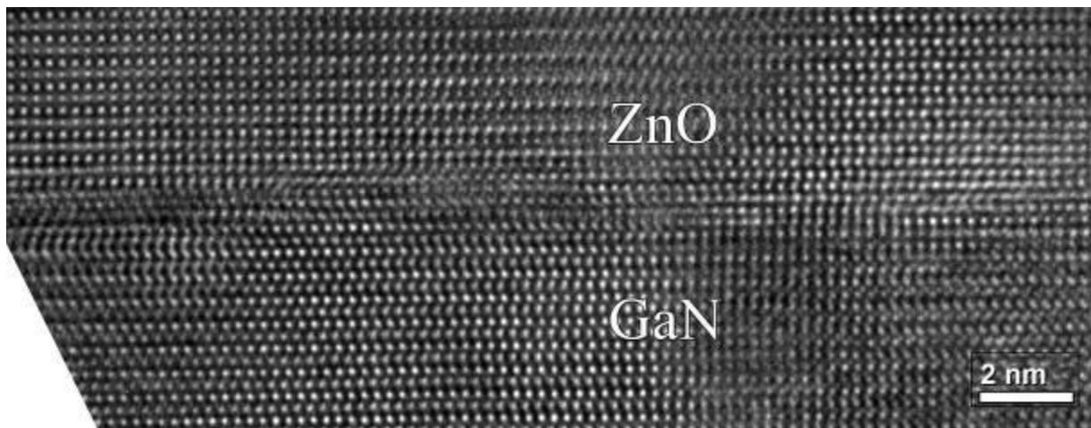
**Figure 3.** Aberration-corrected high-resolution TEM image showing an ALD grown ZnO on GaN.
