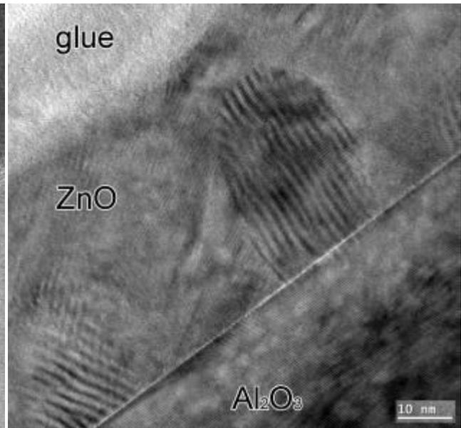
**Figure 2.** BF TEM image of ZnO deposited on (0001) Al<sub>2</sub>O<sub>3</sub>
