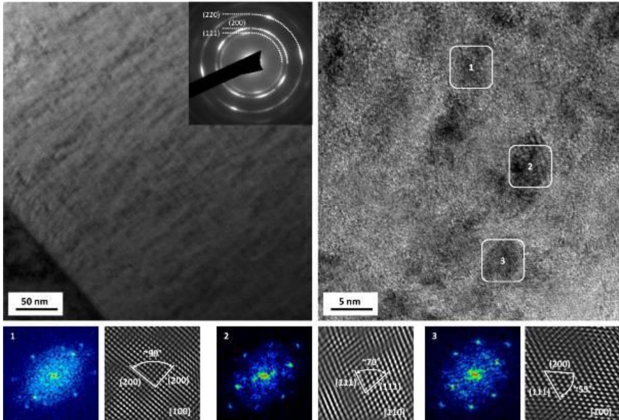
**Figure 1.** Bright field image a) and HRTEM image b) of the cross-section through TiSiN coating, with FFT patterns along with inverse FFT images. The SAED pattern is included in the figure a).
