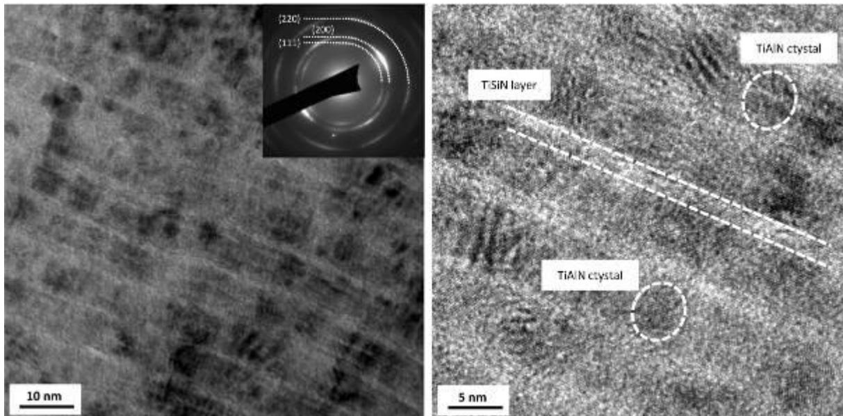
**Figure 2.** Bright field image along with the SAED pattern a) and HRTEM image b) of TiSiN/TiAlN coating
