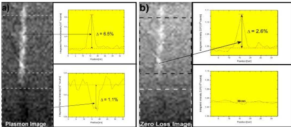
**Figure 2.** (a) Image of the Plasmon signal (energy window: 12-18 eV) extracted from the individual electron-energy loss spectra and corresponding profiles across boxed regions. Note the contrast inversion compared to the HAADF detector signal in Fig.1. (b) Image of the zero loss peak (ZLP) (energy window: 5 eV) extracted from the individual electron-energy loss spectra and corresponding profiles.
