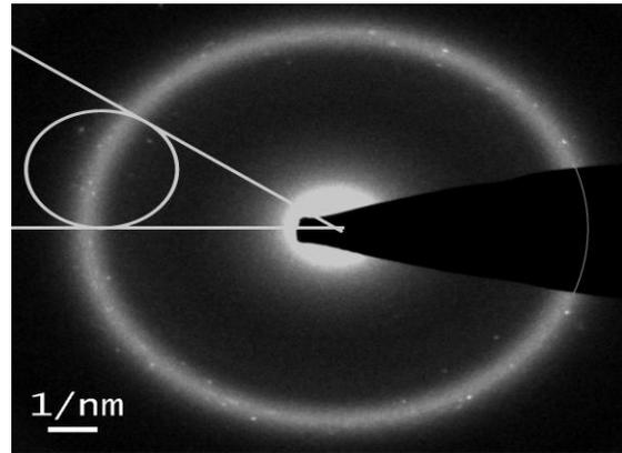
**Figure 4.** Diffraction pattern with marked objective aperture lying on the diffuse ring of the amorphous phase and containing spots of the nanocrystals
