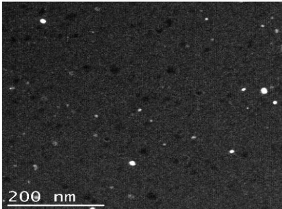
**Figure 3.** Dark field image of the evaluated area (same area as in Fig. 2), showing bright but also dark nanocrystals.
