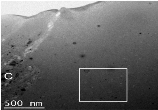
**Figure 1.** Amorphous phase with the evaluated area and a crystalline area C on the left side
