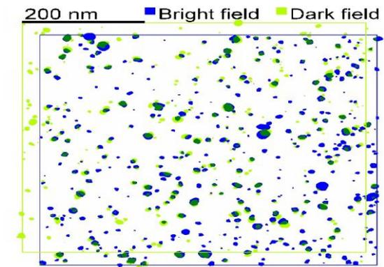
**Figure 5.** Combined mask image of the segmented bright field and dark field images of the nanocrystals
