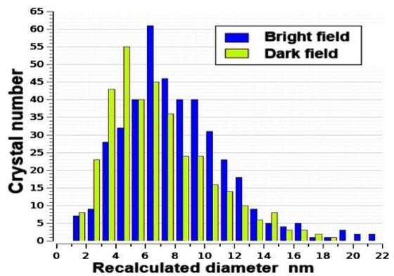
**Figure 6.** Frequency - diameter graph of the crystals for both the bright and the dark field evaluation
