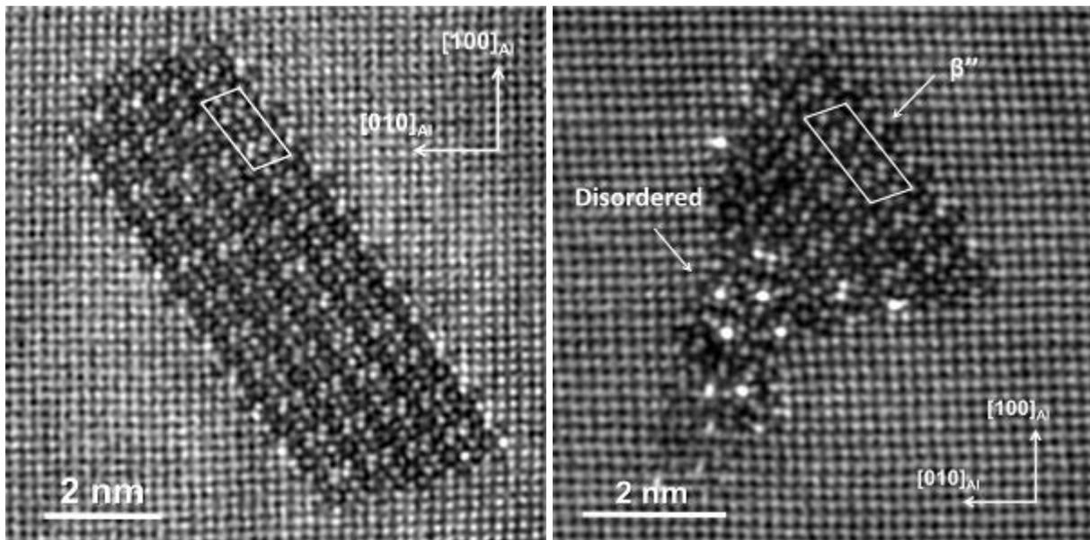
**Figure 1.** HAADF-STEM images from  $\langle 100 \rangle_{\text{Al}}$  direction for (left) Cu-containing  $\beta''$  precipitate and (right) Cu-containing  $\beta''$ /disordered precipitates. In these images, periodicity shorter than  $1.5\text{\AA}$  are filtered out with a circular band pass mask.
