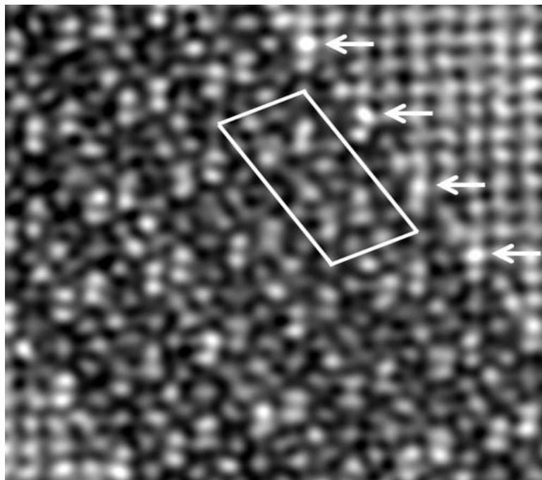
**Figure 2.** Enlarged part of the left image in Figure 1. Arrows indicate possible replacements of Cu atoms at Si positions in the interface of the  $\beta''$  precipitate, which was determined due to the atomic number contrast. The  $\beta''$  unit cell is drawn in the figure.
