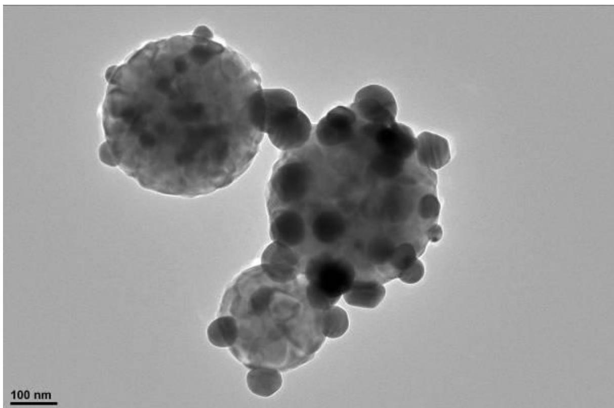
**Figure 1.** TEM image of Ag-TiO<sub>2</sub> nanoparticles.
