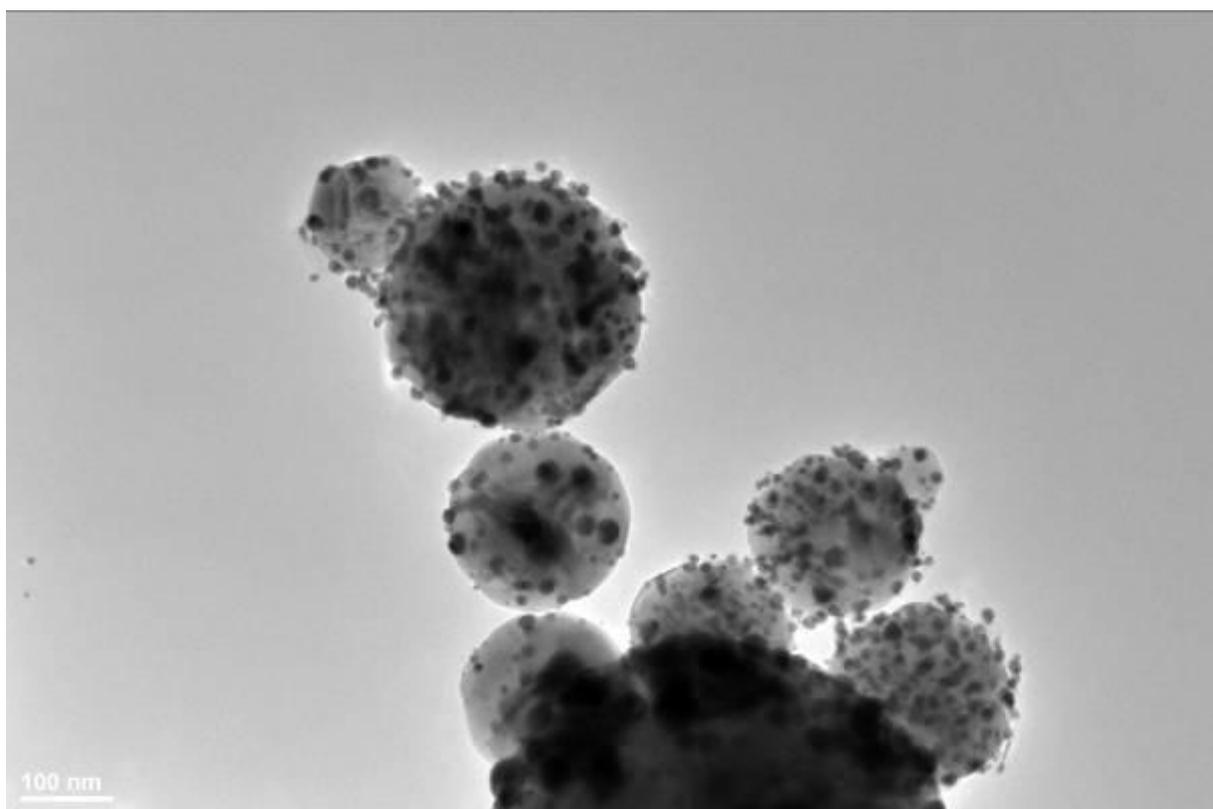
**Figure 2.** TEM image of Au-TiO<sub>2</sub> nanoparticles.
